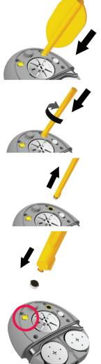
4. **Firmly push** the tip of the removal tool into the middle of the microphone protector.
