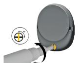
1. If the battery cover is locked, turn the lock screw anticlockwise to unlock it.
